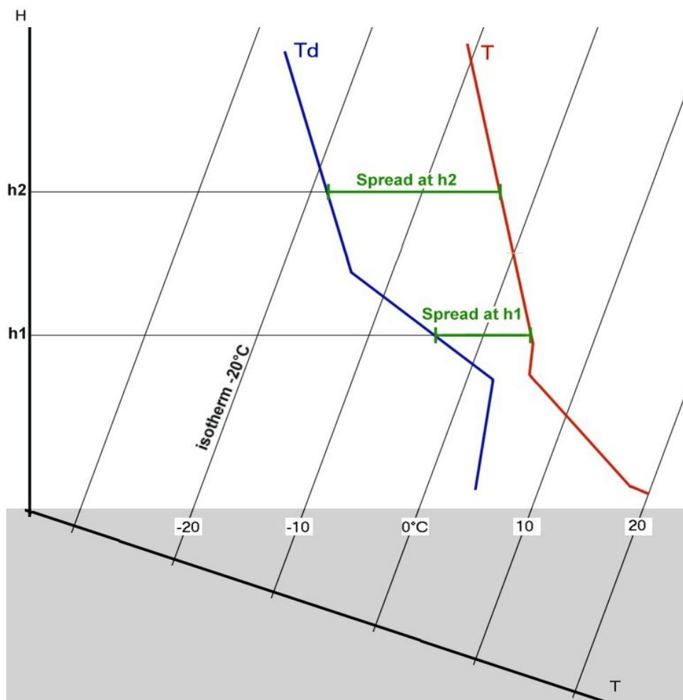
Figure 1: principle of an emagram. Only some isotherms and isobars  $h_1$  and  $h_2$  are shown.
