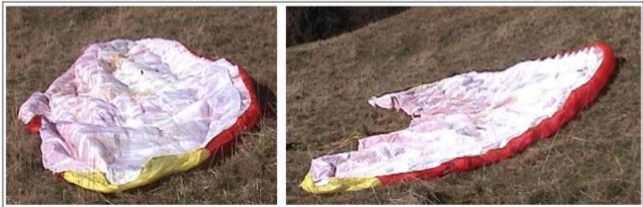
Figure P7: Positioning of the wing on take off. Left - wing is laid out sailing straight (unfavorable). Right - wing is laid out in an arc (favorable).
