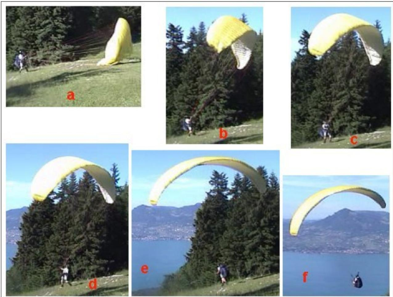
*Figure P13: Reverse take off. The pilot inflates (a), raises (b) and (c) controls the wing before (d) turning and checking the glider and airspace and then (e) leaning forward and running. Once away from the slope, he finally settles into the harness (f).*
