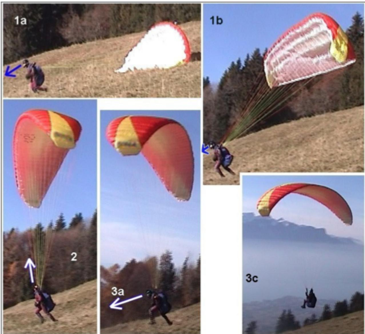
Figure P10: 3 phased take off. 1a = inflation, 1b = lifting the wing, 2 = control, 3a = acceleration, 3c = sitting in the harness. The arrow shows the direction of sight.
