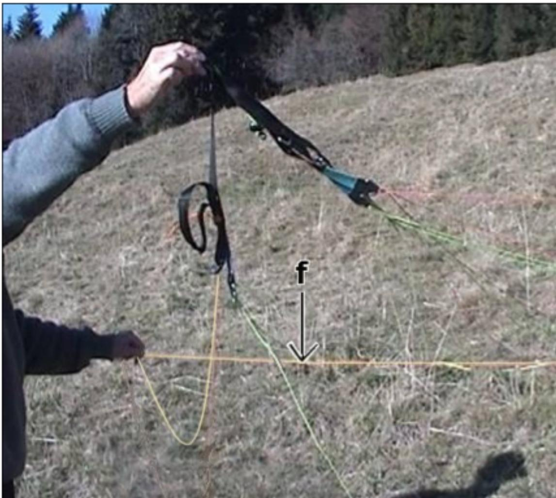
Figure P8: disentangling the brake lines (f).
