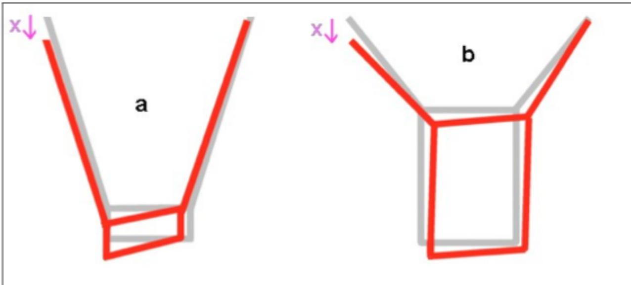
Figure C24: Influence of the gap between runners, not the principle adjustable waist belt. a = small gap, b = larger gap, x = lateral oscillation amplitude transmitted through the veil lifts, z = axis of plate rotation (axis of moment of force couple) holding the twist.
