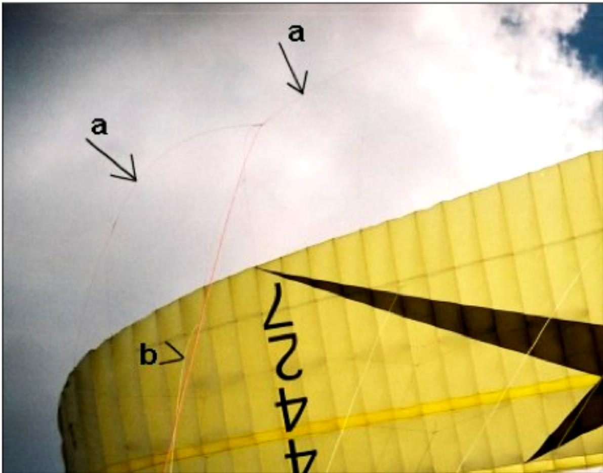
Figure C20: a = left brake lines curved backwards, b = D lines slightly curved.
