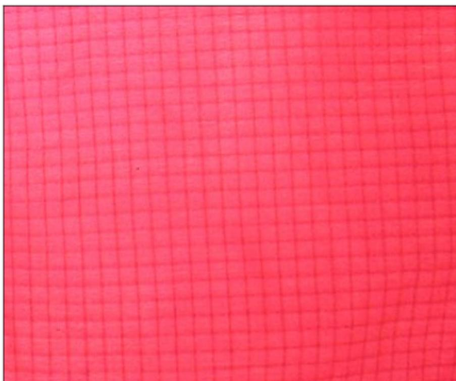
*Figure C2: ripstop fabric with finely squared appearance. One direction is called the weft, the other (perpendicular) is called the warp.*
