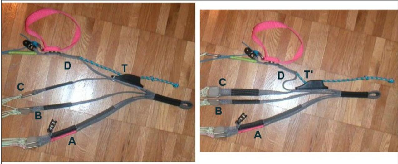
Fig C18: Glider equipped with trim-tabs.  $T$  = inactive and  $T'$  = active. Riser groups A to C are not affected by the trim-tabs. When the trim-tab is engaged, the lower part of the D risers folds and shortens.
