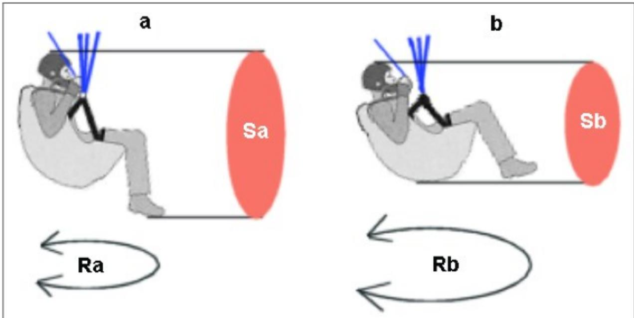
Figure C27: Influence of the pilot's position on the drag and the tendency to twist. a = sitting, b = lying down, S = surface projected to the wind by the pilot & harness, R = moment of torque (rotational power) of pilot and harness inducing a twist.
