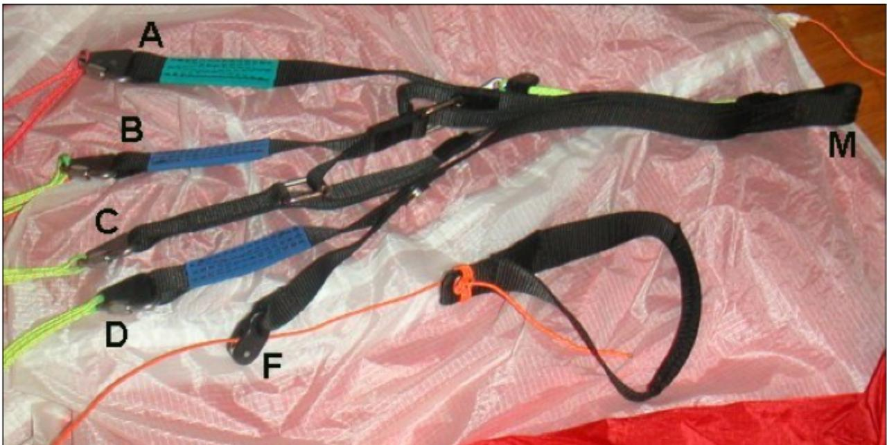
Figure C12: 4 Risers A to D. F = small brake handle (control). M = end loop that attaches to the harness.
