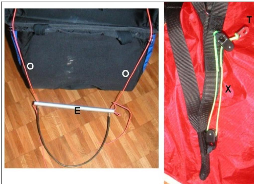
Figure C14: O = cord connection. E = stirrup.
