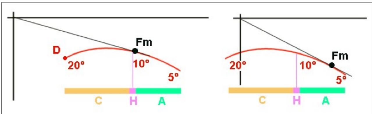
Figure C17: Polar curve of a paraglider in still air (left) and a 25km/h headwind (right). D = stall. C = flight range with the brakes. H = range of "hands up" flight. A = area of flight with the accelerator. Fm = maximum glide ratio.
