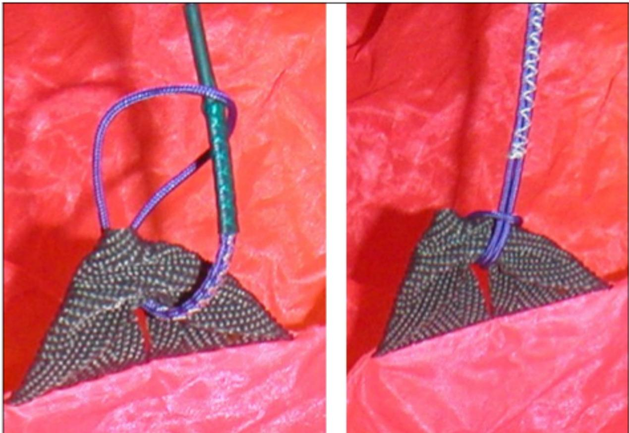
*Figure C10: Fixing a line to the underside of a wing.*
