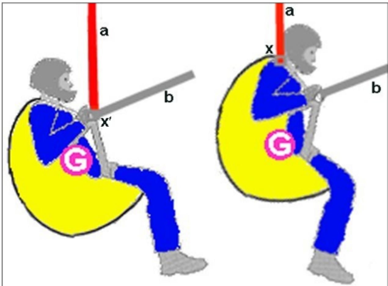
Figure C29: Influence of the positioning of attachment points in order to force the pilot into an upright position on deployment of the rescue chute. *a* = rescue risers, *b* = paragliding risers, *G* = center of gravity, *x* = attachment to karabiners resulting in a seated landing, and injury, *x* = attachment to the shoulder straps of the harness resulting in a better vertical position pilot.
