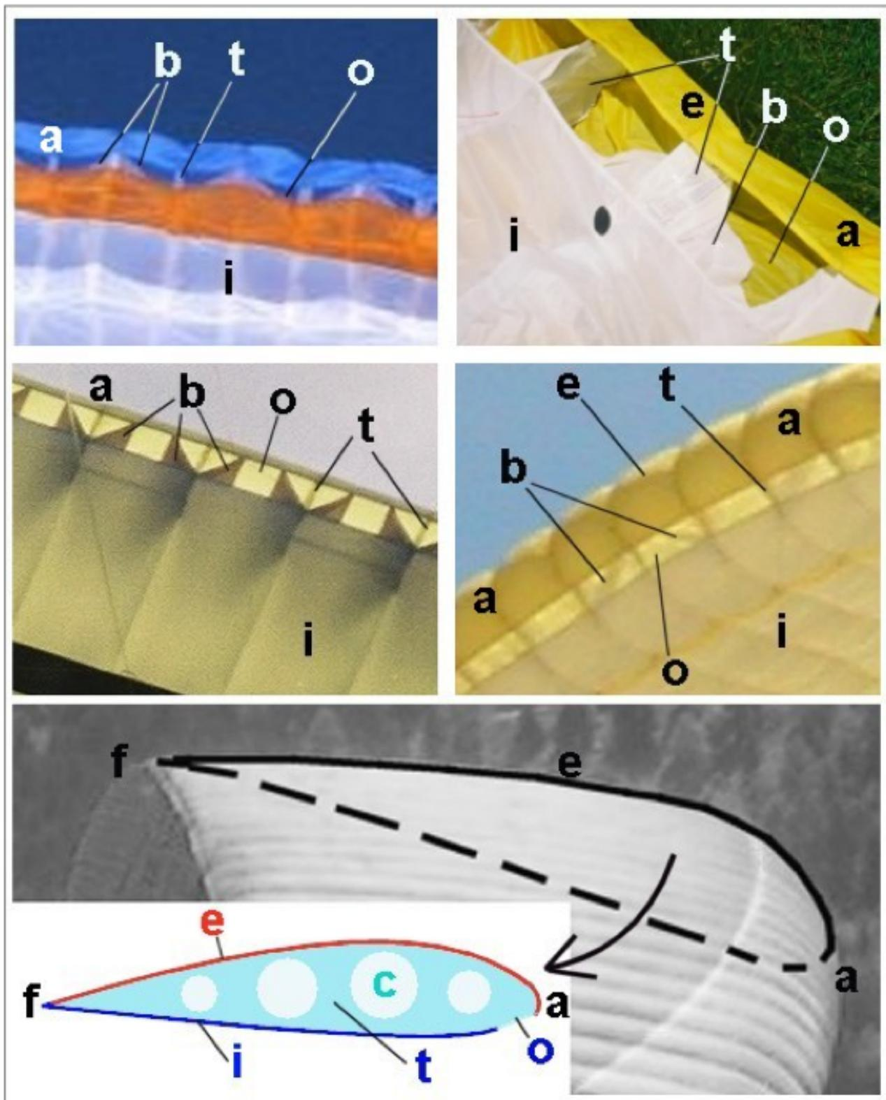
Figure C3: Structure of a wing: a = leading edge, f = trailing edge, e = upper surface, l = lower surface, t = cell walls, o = cell openings, b = diagonal bracing, c = hole (vents) in cell walls.
