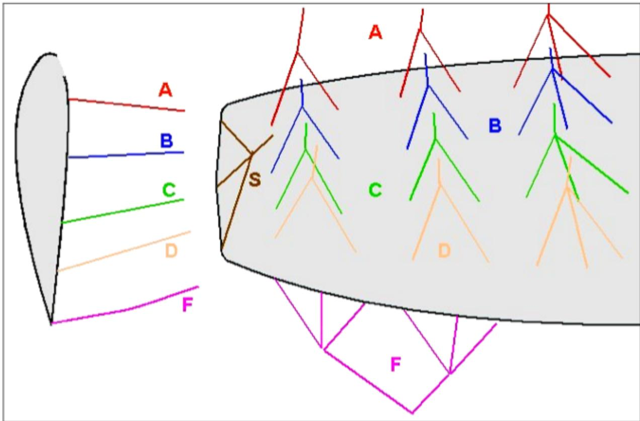
Figure C7: The groups of lines and sample line plan (underside view). Groups A to D on the underside. F = control lines (brakes). S = suspension of stabilizer.
