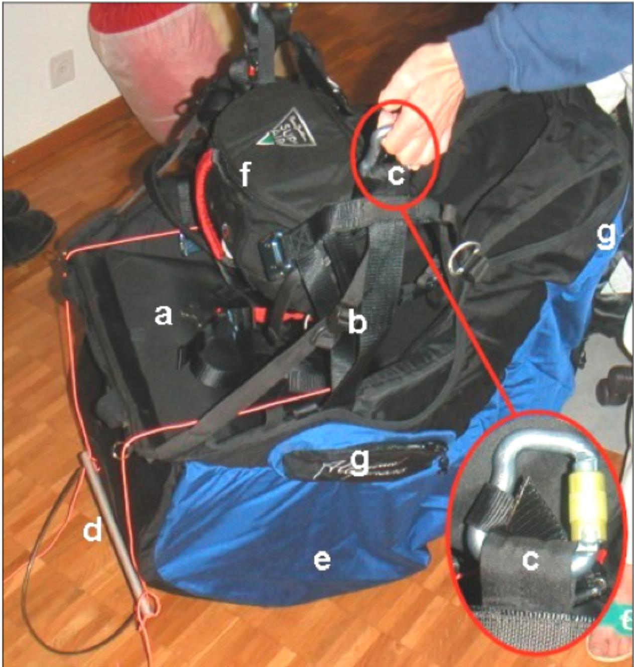
Figure C21: Example of harness with airbag, a = lower (rigid) seat, b = side straps converging on the karabiner (c). s = speed bar, e = back protection, f = rescue parachute (in pouch), g = storage pockets, side and rear.
