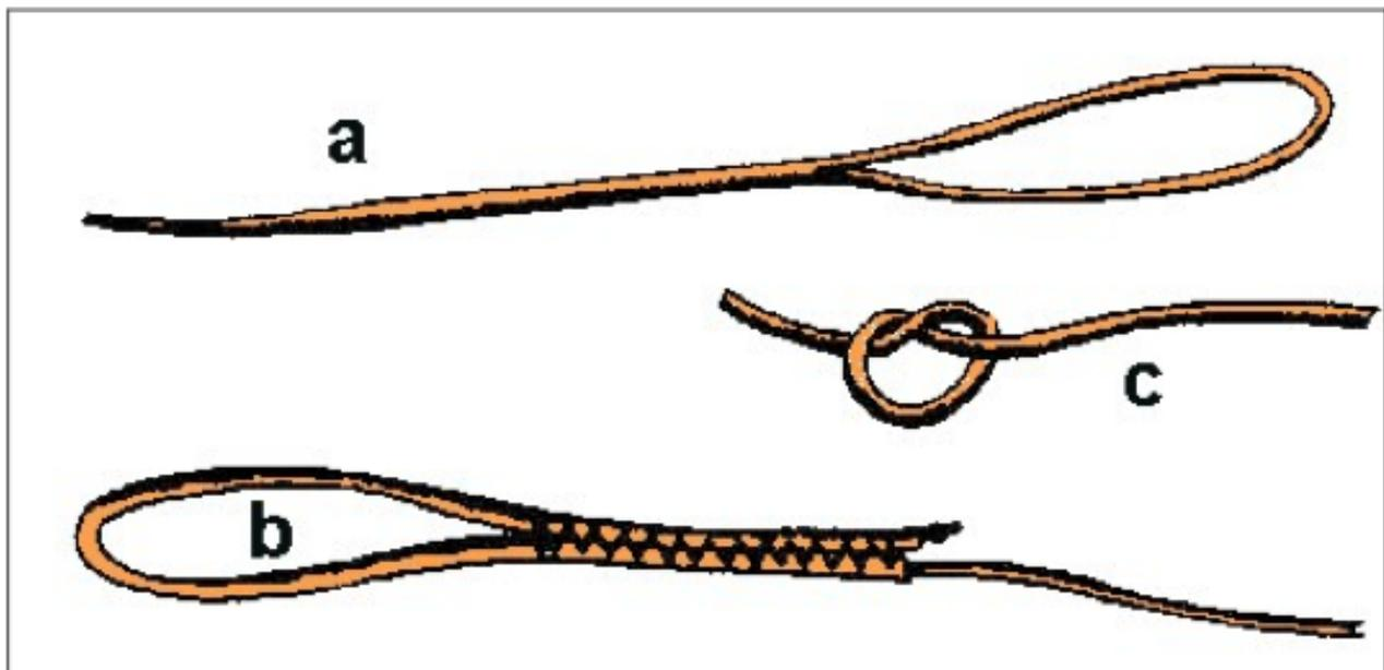
Figure C9: a = splice, b = sewing, c = knot.
