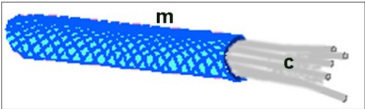
Figure C8: structure of a liner. m = mantle, c = core.
