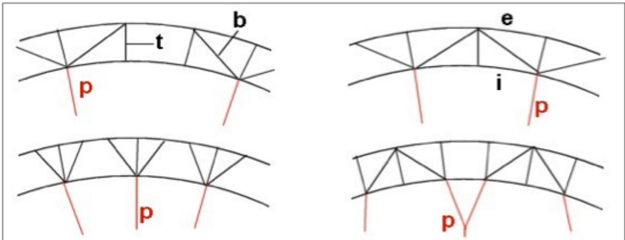
Figure C4: Schematic side view of a wing with illustrating different kinds of arrangement of vertical walls and diagonal bracing. *t* = cell walls, *b* = diagonal bracing, *p* = lines, *e* = upper surface, *i* = lower surface.
