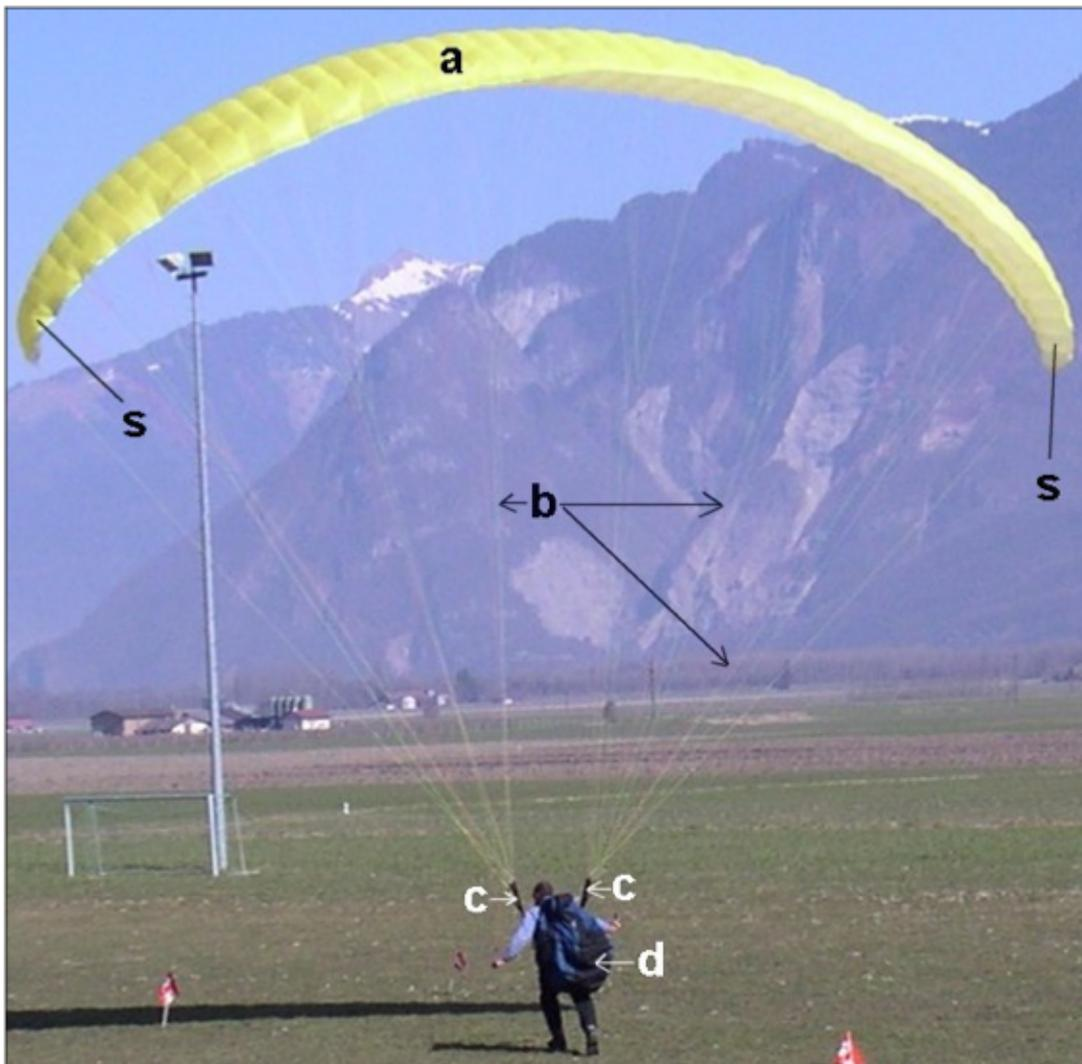
Figure C1: the 4 main parts of a paraglider. a = wing, b= lines, c = risers, d = harness, s = stabilisers.
