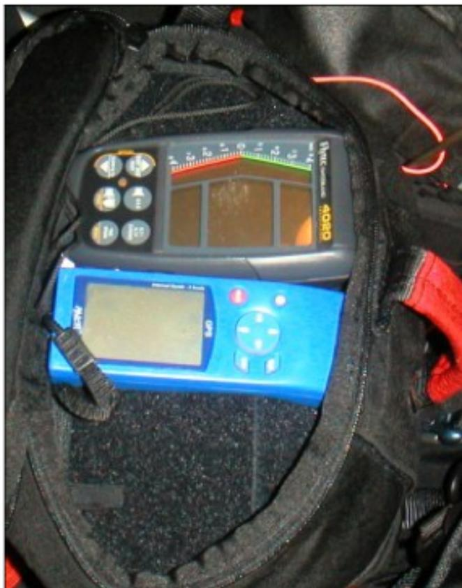
*Figure C32: A collection of flight instruments: an altimeter and variometer (above), and a GPS tracker (below). Both instruments are shown placed on the outer pocket of a ventral reserve parachute.*
