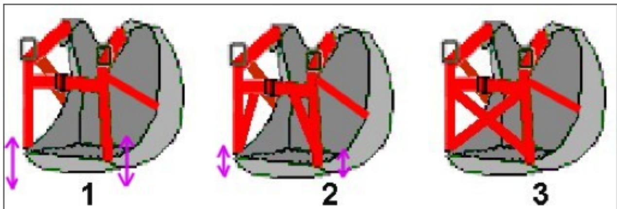
Figure C23: 1 = no cross bracing, 2 = ABS (anti balance system), 3 = lattice (or cross braced) harness. In turbulence, the arrows represent the amplitude of lateral oscillating movements.
