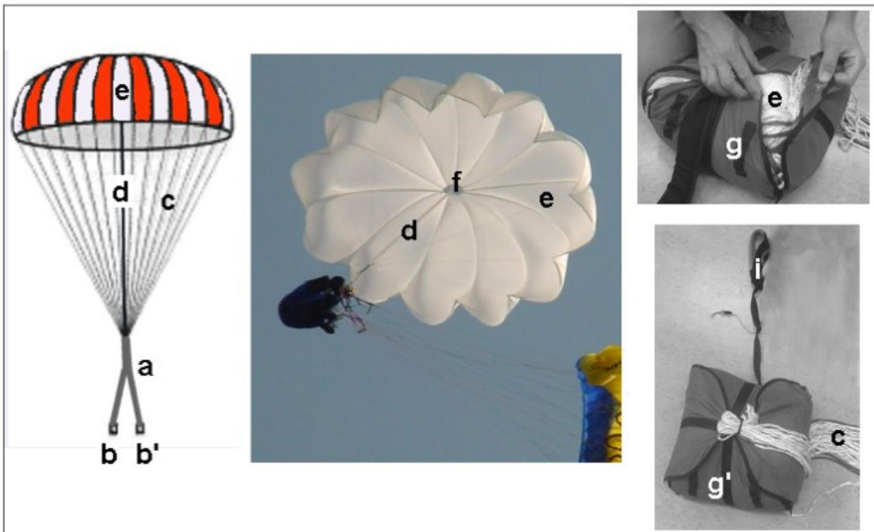
Figure C28: Elements of the emergency parachute. a = risers (sling) branching symmetrically, b = large link attachments with trapezoidal quick links attached to the harness (usually to the shoulder straps), d = central suspension line, c = finer lateral suspension lines, e = parachute, f = vent (opening), g = cover (internal container), g' = internal container when closed, i = container strap and handle for its release from the pouch (external container) in the harness.
