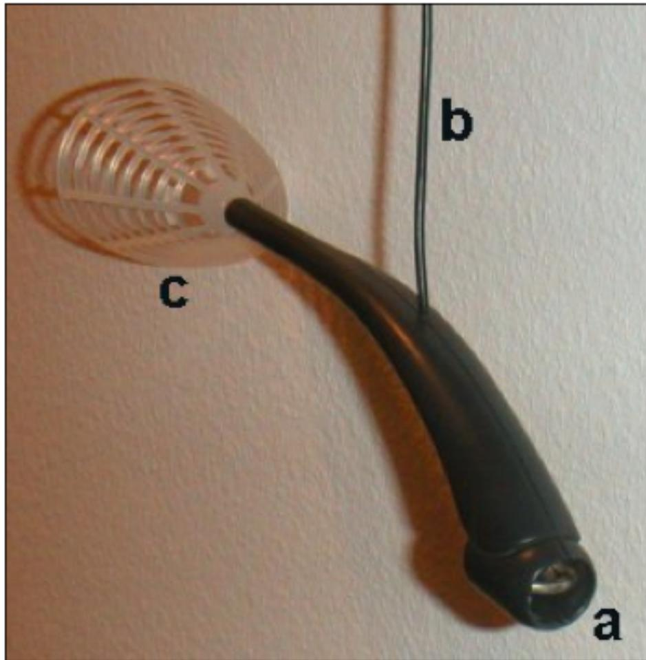
*Figure C33: Anemometer. a = anterior opening in which is housed a propeller, whose speed of rotation depends on the wind. b = wire for attaching the device to the harness and containing the wires used to receive the signal. c = tailplane to provide directional stability of the instrument.*
