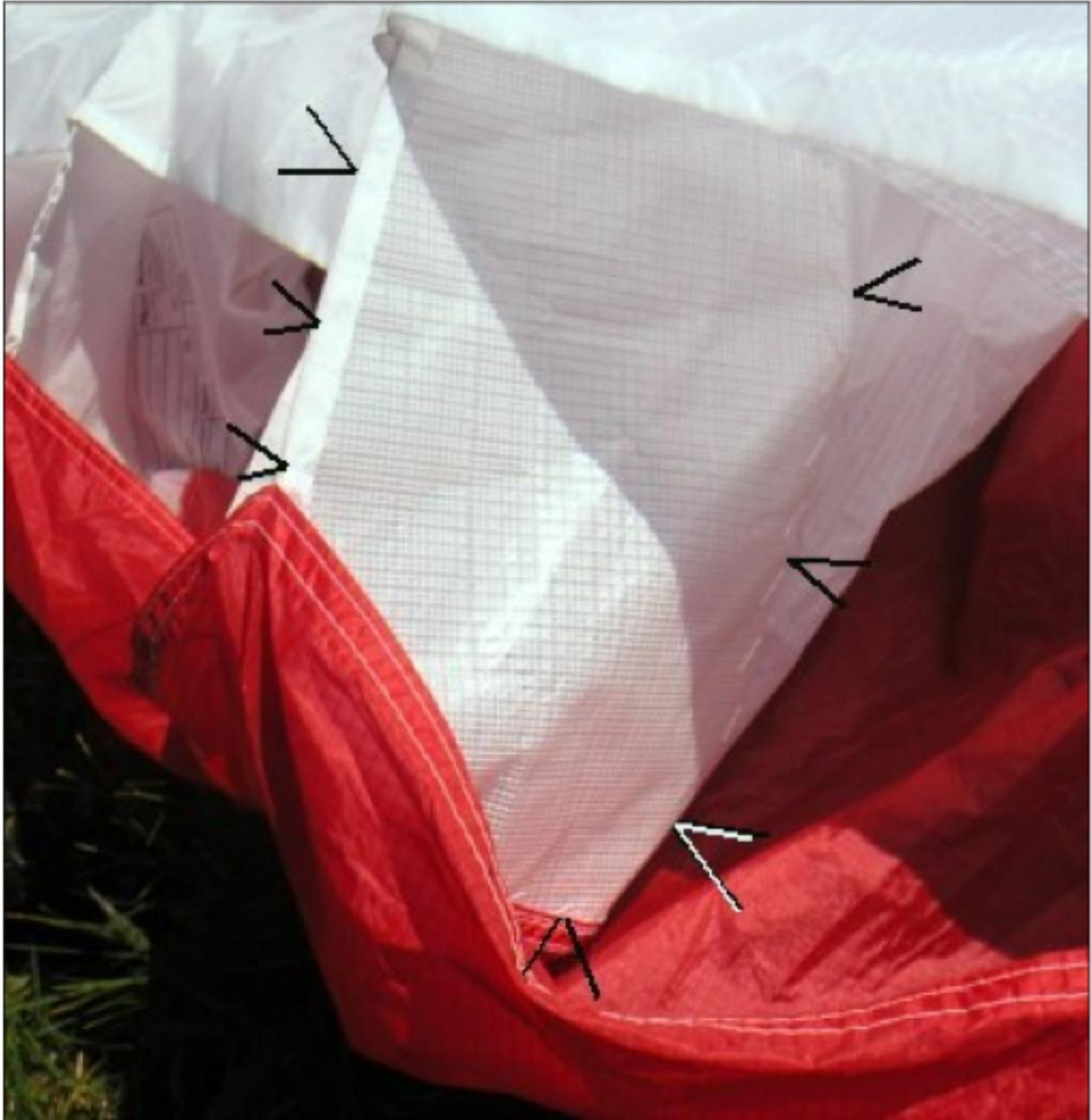
Figure C6: fabric reinforcements coated with Mylar.
