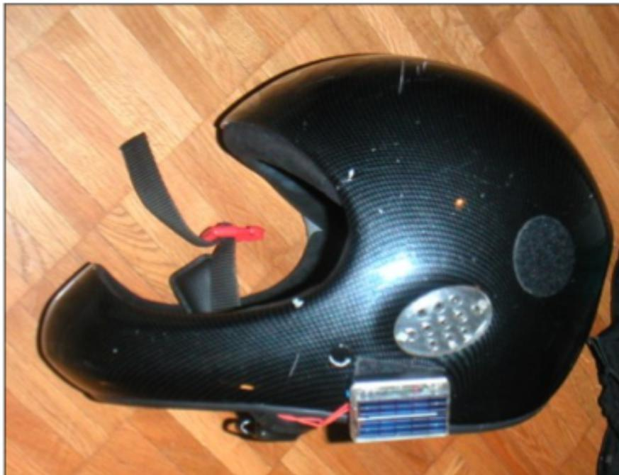
*Figure C31: Paragliding helmet. The small device with solar cells, placed at the bottom edge and side of the helmet is a small acoustic variometer (without batteries): light and efficient.*
