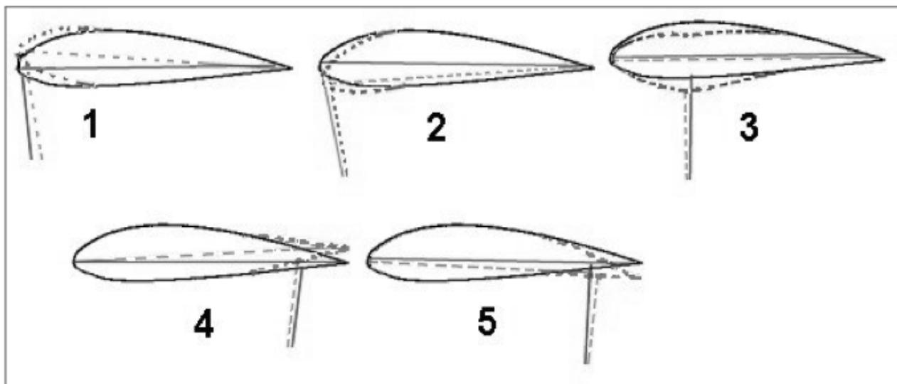
Figure C11: Dotted line, change in the angle of attack when the length of group A, B or D lines change. Solid line, the angle of attack before modification.
