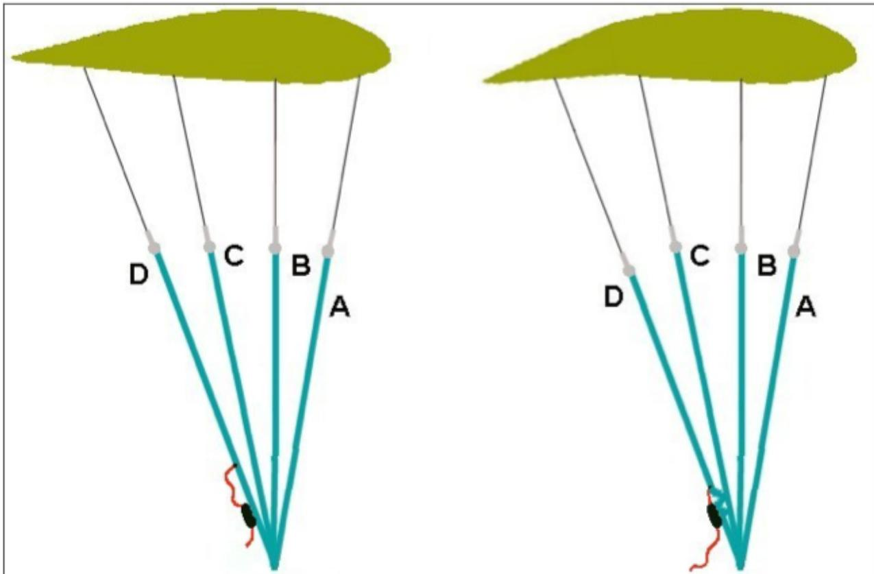
Figure C19: Schematic of a glider with trim-tabs inactive (left) and engaged (right).
