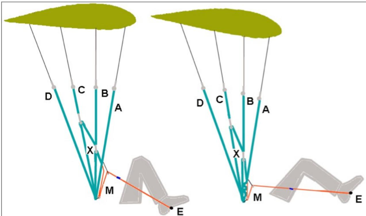
Figure C16: Schematic of a riser before (left) and after (right) application of the foot control. On the right, the systematic, progressive shortening of the risers D to A. X = differential in shortening of the risers. M = multiplier accelerator. E = accelerator bar.
