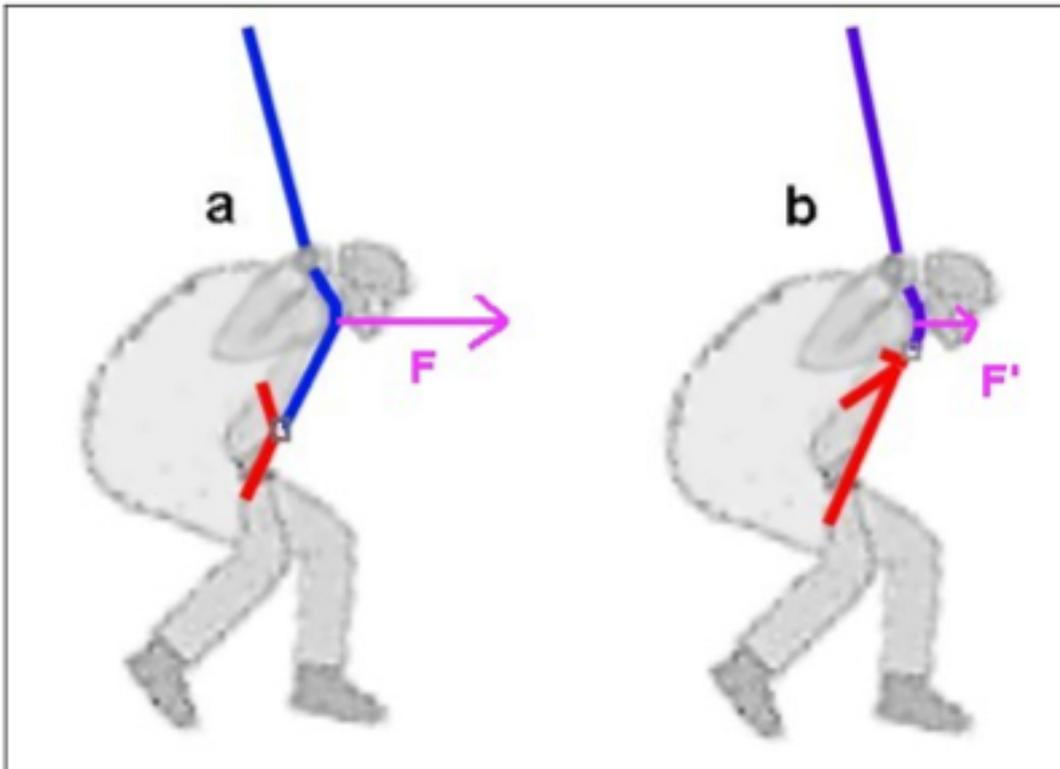
Figure C26: Influence of the height of the position of the karabiner on the pilot's take-off position. a = karabiner located low, b = karabiner located high.  $F$  and  $F'$  = moment of torque at pilot's shoulders.
