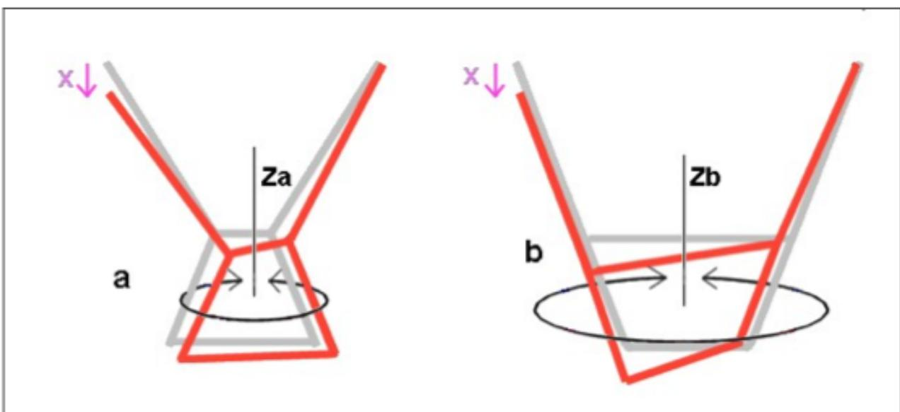
Figure C25: Influence of the height of karabiners. a = low karabiners, b = high karabiners. , X = amplitude of lateral oscillation transmitted by wing through the risers.
