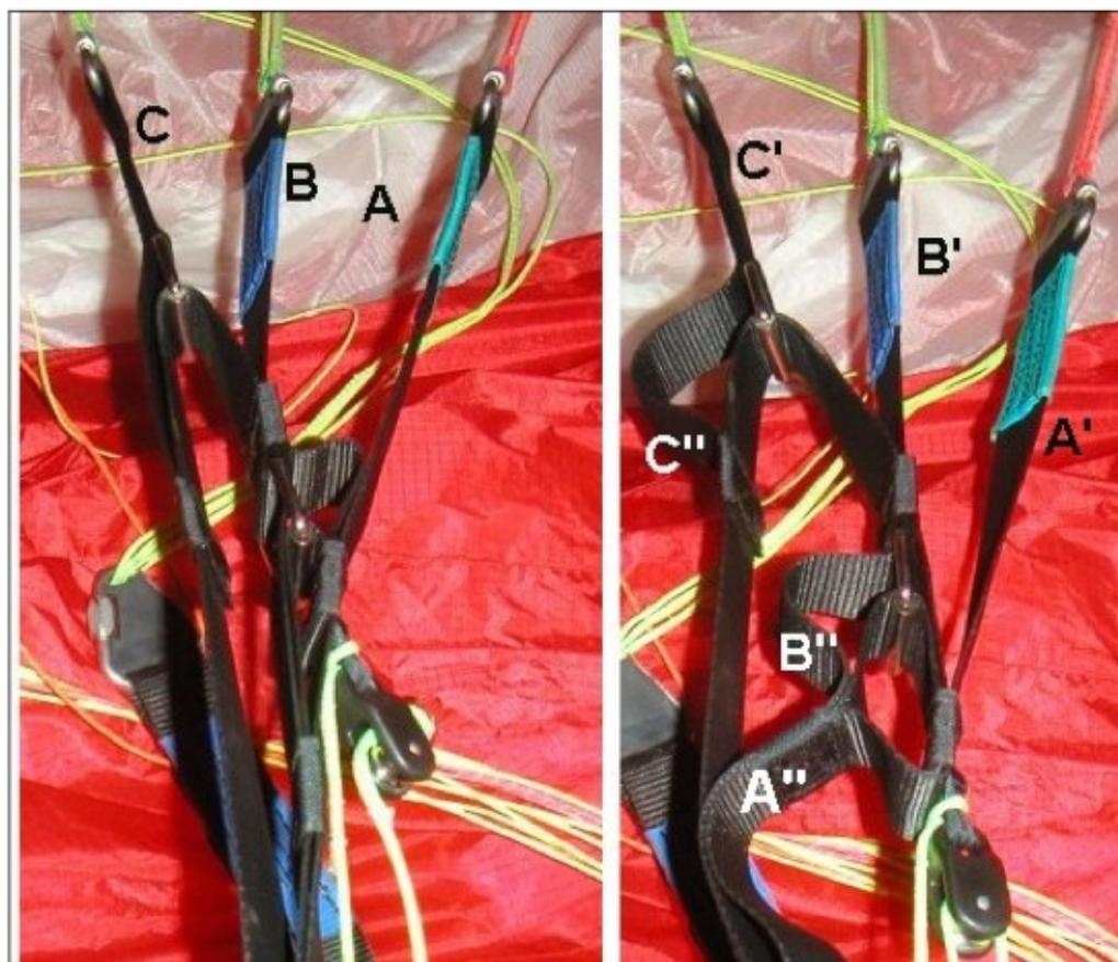
Figure C15: Accelerator system, before (left) and after (right) application. Shortening of A, B, C to new positions of A', B' and C'. The bottom riser is pleated A'', B'', C'' after application of the accelerator.
