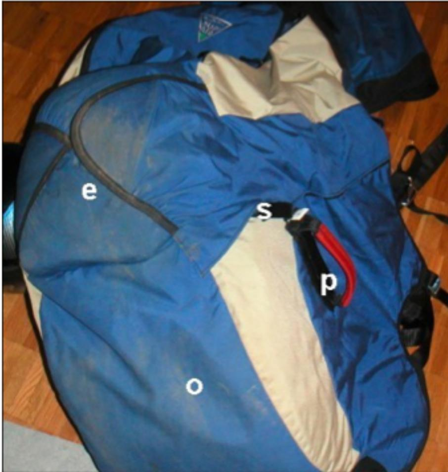
*Figure C30: Example of a exterior, read pouch for the reserve parachute, attached to the harness. e = external pocket, o = foam fall protection, s = connecting strap between the internal reserve pouch (hidden in the external pouch) and p = emergency handle.*
