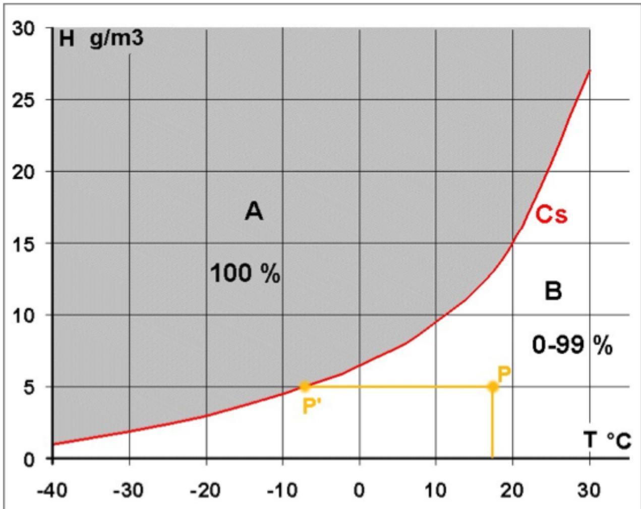
Figure M12: Relationship between temperature and humidity.  $C_s$  = saturation curve, where condensation occurs. A = area of 100% humidity and fog/mist. B = clear air with a humidity ranging from 0-99%.
