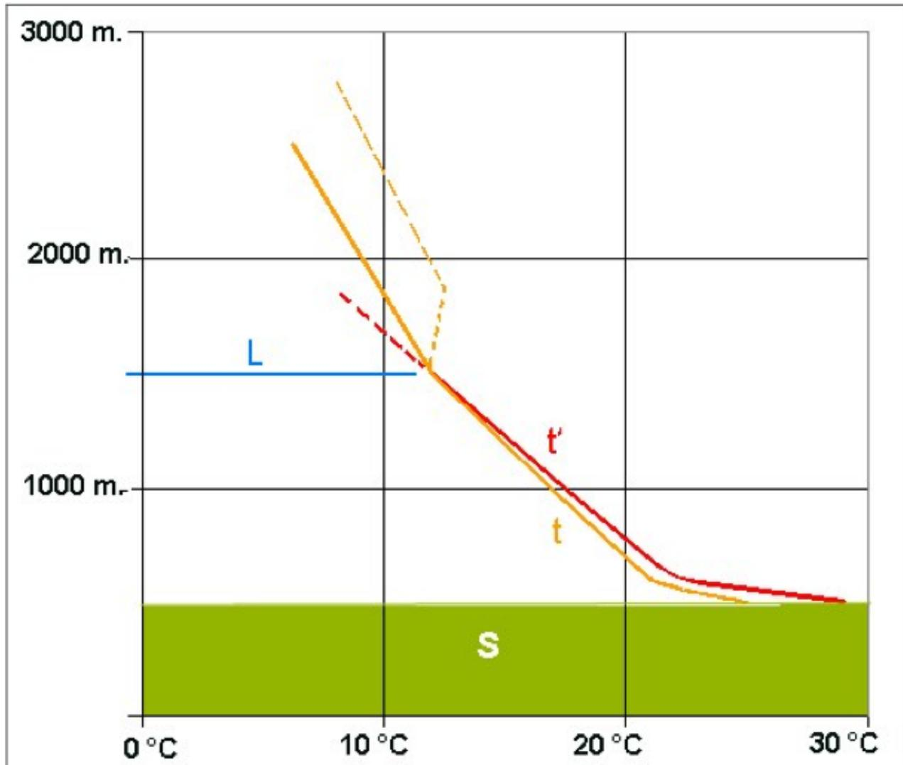
Figure M10: Graph comparing the temperatures of the ambient air compared to air in the thermals, depending on altitude. L = upper limit of the convective layer. t = static temperature curve. t' = rising thermal temperature curve. The values correspond to those of figure M09.
