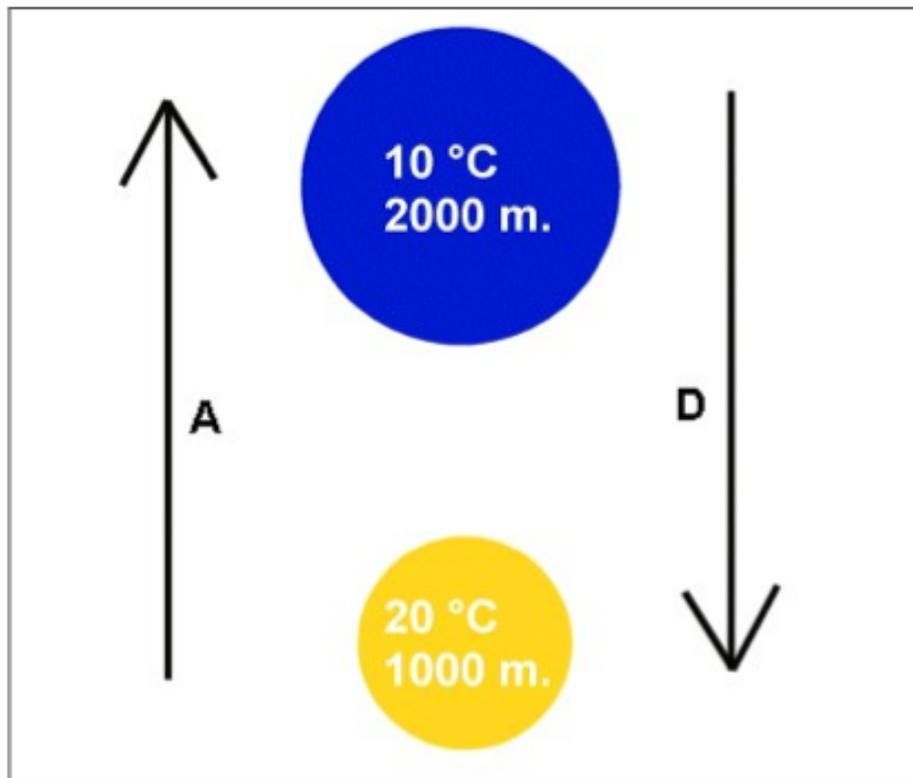
Figure M05: Lapse rate. A = mass of air rises, expands and cools  $1^{\circ}\text{C}/100\text{m}$ .
