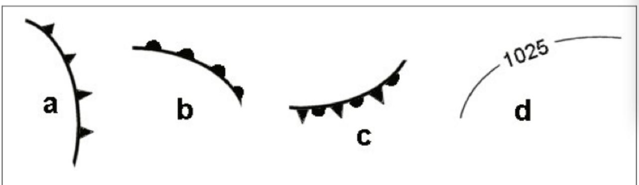
Figure M31: Some symbols used in the synoptic charts, a = cold front, b = warm front, c = occlusion, d = isobar at 1025hPa.
