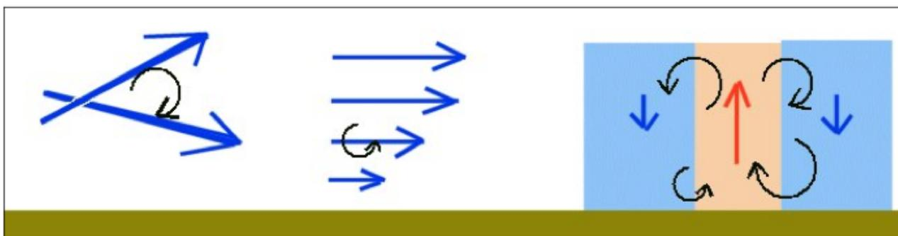
Figure M26: shear turbulence (2 figures on the left) and thermal right figure).
