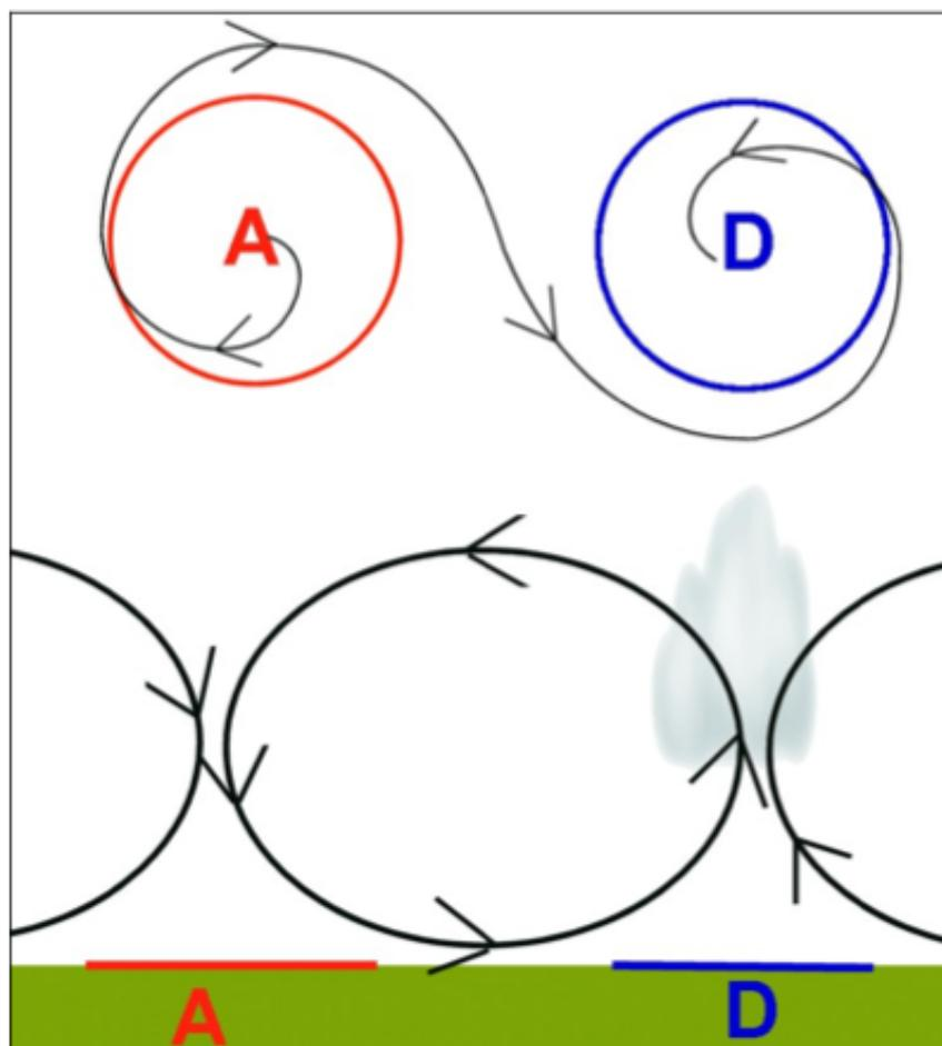
Figure M22: 3 air movements around the centers of action: Vertical (descending in anticyclones, rising in depressions), rotary (around Action Centers), horizontal (spiraling away from high pressure, and spiraling towards low pressure). A = Anticyclone. D = Depression.
