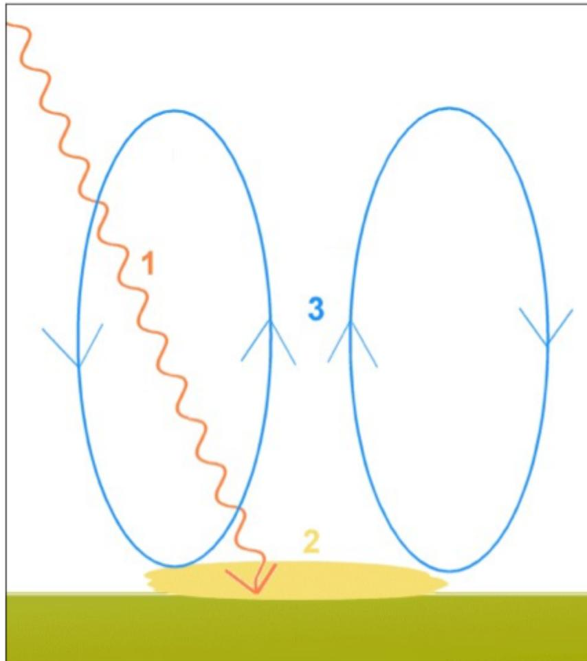
Figure M04: Indirect warming of the atmosphere in 3 phases: (1) solar radiation through the air, (2) conduction into a thin layer of air to ground, (3) convection.
