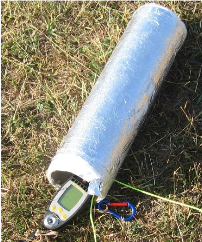
Figure 1: The JDC GEOS 11 device with the tube protecting against heating from direct sunlight.
