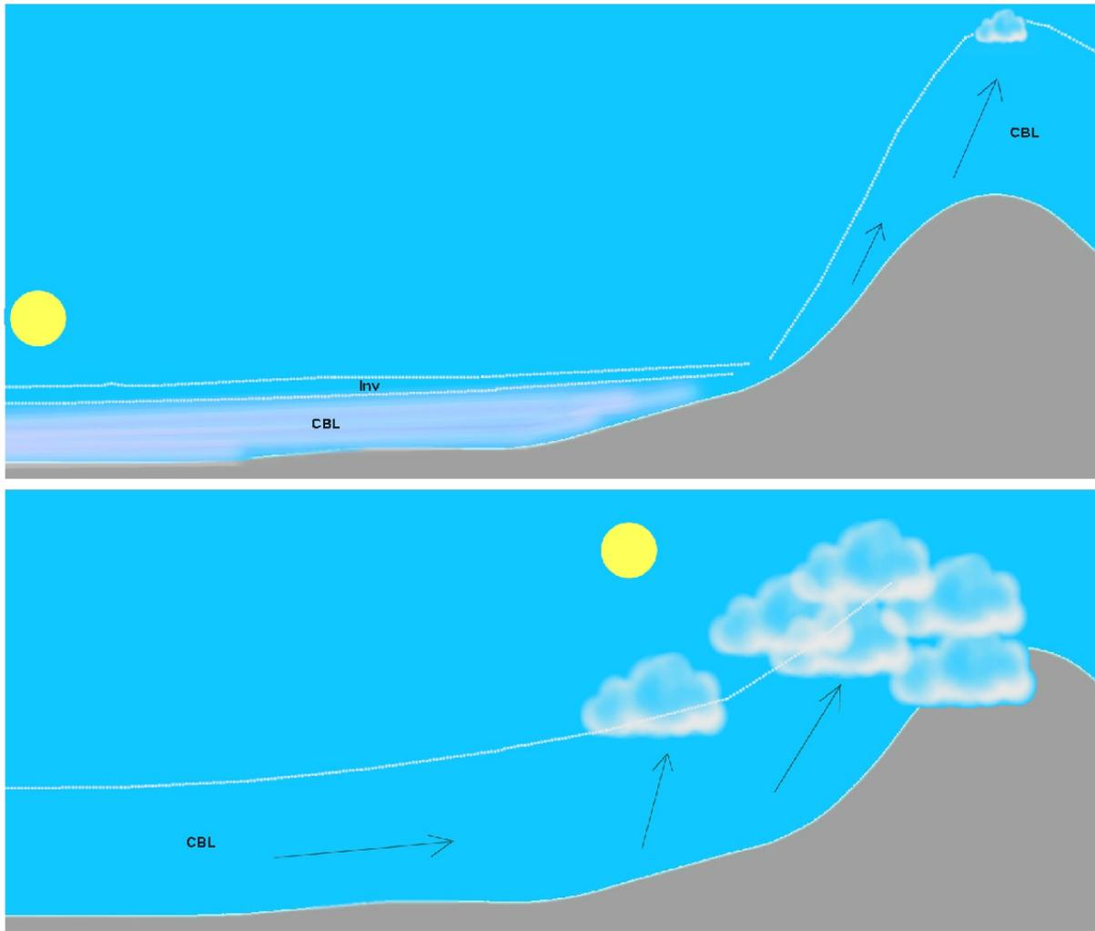
Figure 14: Hypothetical explanation of the cloudbase's lowering in front of Dhauladhar as the day progresses. CBL = convective boundary layer. Inv = temperature inversion.
