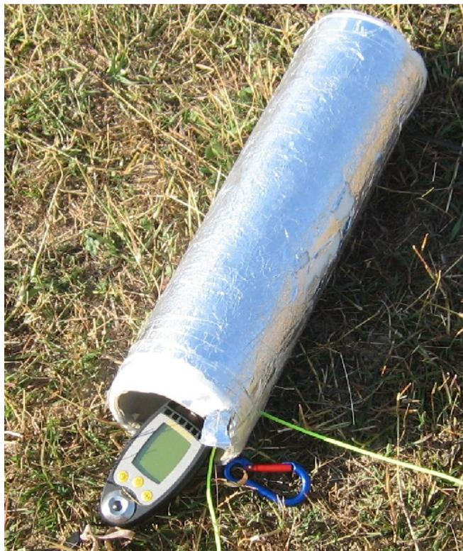
Figure 1: The JDC GEOS 11 device with the tube protecting against heating from direct sunlight.
