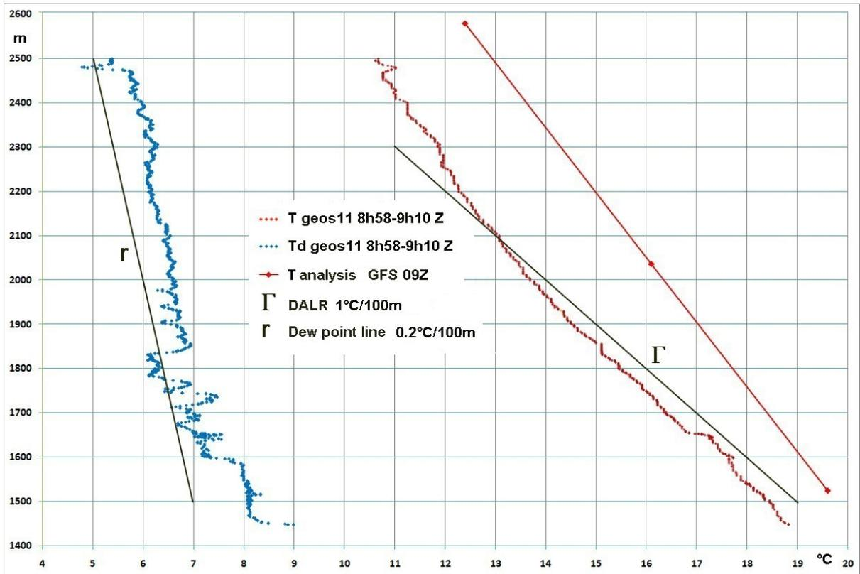
Figure 6: The measured profile (temperature and dew point) of the final descent.
