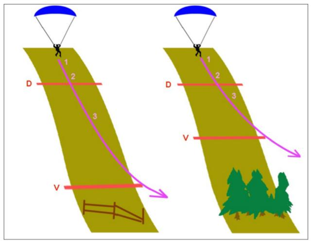
Figure P6: take off site. D = decision line. V = point of no return. 1, 2 and 3 = stages of take off.
