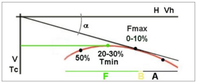
Figure P15: Polar curve of a paragliding wing.  $A = range requiring use of the accelerators system. \alpha = glide angle for maximum glide ratio. Fmax = maximum glide ratio, Tmin = minimum sink rate. H = distance, V = loss of altitude, Vh = horizontal velocity, Tc = rate of fall. % = Percentage of braking. F = range requiring use of brakes. B = range of "arms up" flight.$
