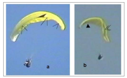
Figure P25: B line stall (a) and asymmetrical collapse (b). Arrow = single fold on the underside at the points of attachment of the B lines. Double arrow = closure (collapse) of left side of the wing. Arrow = compensation to maintain direction by the applying right brake.
