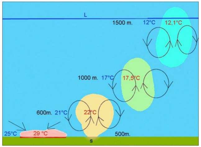
Figure M09: Evolution of the temperature of the air in a rising thermal bubble. The upper limit = the convective layer.
