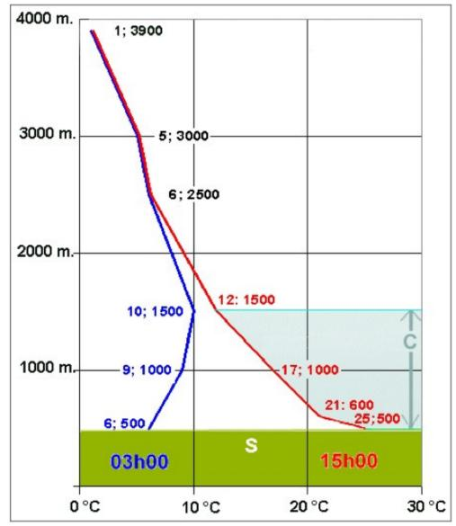
Figure M08: emgrams typical of a clear and calm night (blue) and the following sunny afternoon (red) with the same general weather situation. S = ground (soil). C = convective layer (1°C/100m).
