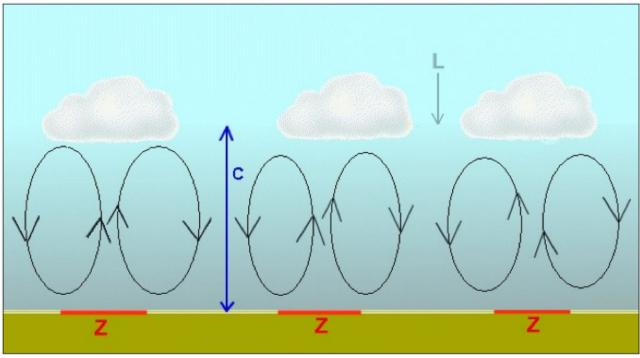
Figure M03: Movements currents. C = convective layer (foggy). L = upper limit of C. Z = efficient heat sources on the ground.
