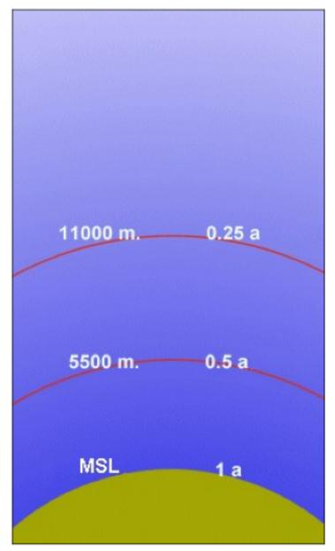
Figure M02: decrease in atmospheric pressure with altitude. Major reference points. MSL = mean sea level = 0 m.
