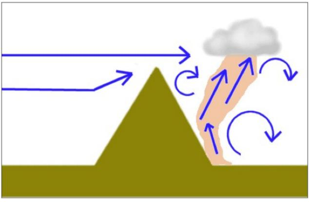
Figure M30: thermal downwind of a relief.
