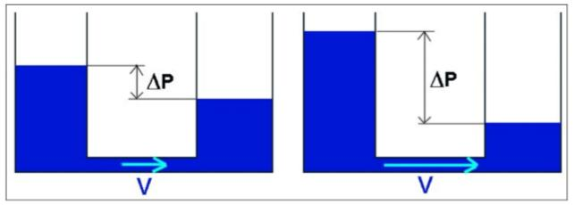
Figure M21: Connecting vessels. Liquid will move from the vessel in which the pressure (height) of the liquid is higher to the vessel where the pressure (height) of the liquid is lower.  $\Delta P$  = differential pressure. V = velocity of the fluid.
