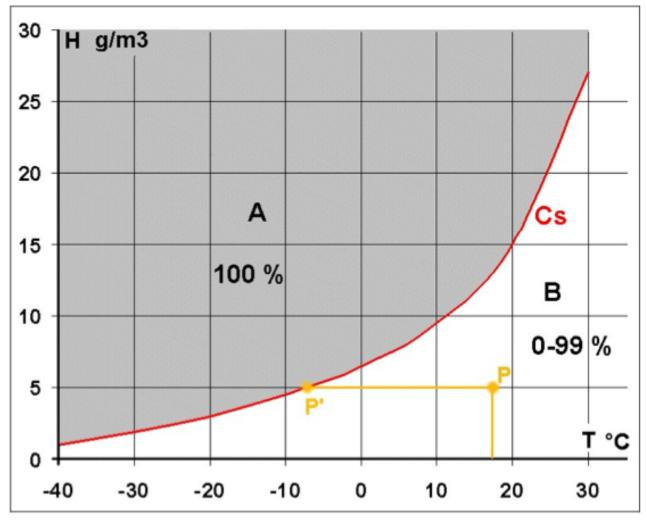
Figure M12: Relationship between temperature and humidity. Cs = saturation curve, where condensation occurs. A = area of 100% humidity and fog/mist. B = clear air with a humidity ranging from 0-99%.
