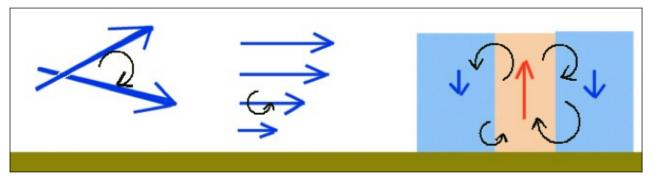
Figure M26: shear turbulence (2 figures on the left) and thermal right figure).
