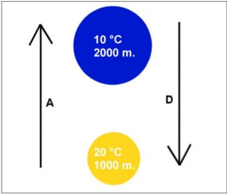
Figure M05: Lapse rate. A = mass of air rises, expands and cools  $1^{\circ}C/100m$ . D = the air mass descends, shrinks and heats  $1^{\circ}C/100m$ .
