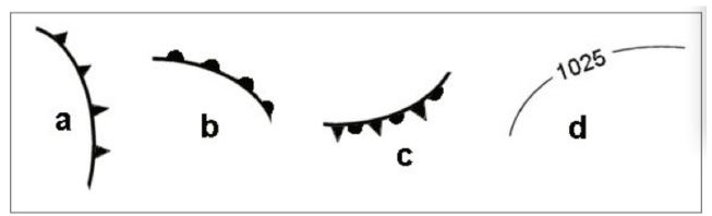
Figure M31: Some symbols used in the synoptic charts, a = cold front, b = warm front, c = occlusion, d = isobar at 1025hPa.
