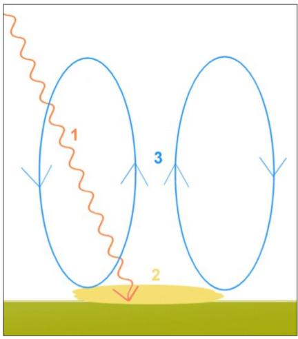
Figure M04: Indirect warming of the atmosphere in 3 phases: (1) solar radiation through the air, (2) conduction into a thin layer of air to ground, (3) convection.
