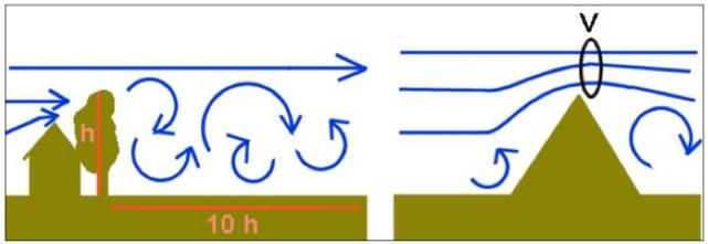
Figure M25: mechanical turbulence
